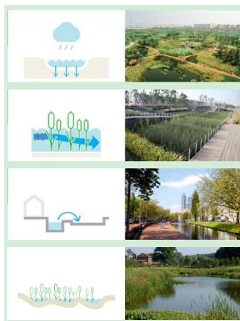
Figure 4.12. Strategies Area B. Top Down: infiltration and retention ponds, natural water purification filters, urban retention areas, expansion of wetlands.
