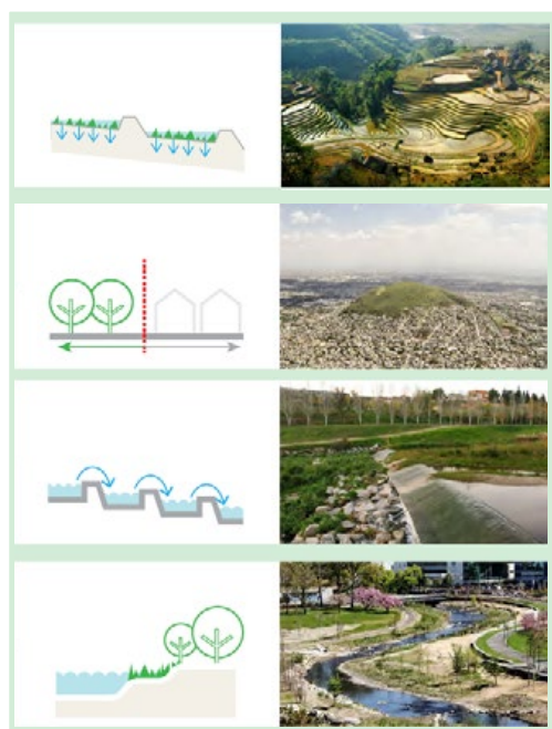
Figure 4.11. Strategies Area A. Top Down: infiltration terraces, limit urbanization, cascading dikes, renaturalisation of ditches.
